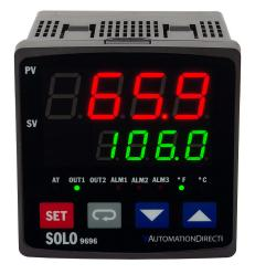
SOLO standard temperature controller, 1/4 DIN, 2-line LED, current, voltage, RTD, thermocouple or event input, 0-10 VDC, 5A SPDT relay, (2) 3A SPST relays output, 100-240 VAC operating voltage, RS-485.
