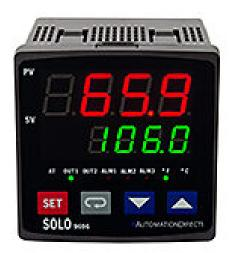
SOLO standard temperature controller, 1/4 DIN, 2-line LED, current, voltage, RTD, thermocouple or event input, 4-20mA, 5A SPDT relay, (2) 3A SPST relays output, 100-240 VAC operating voltage, RS-485.
