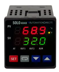
SOLO standard temperature controller, 1/16 DIN, 2-line LED, current, voltage, RTD or thermocouple input, 11-15 VDC pulse, 5A SPST relay, (2) 3A SPST relays output, 100-240 VAC operating voltage, RS-485.
