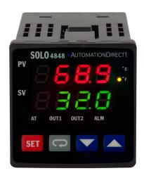
SOLO standard temperature controller, 1/16 DIN, 2-line LED, current, voltage, RTD or thermocouple input, (2) 5A SPST relays, (2) 3A SPST relays output, 24 VDC operating voltage, RS-485.
