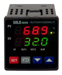
SOLO standard temperature controller, 1/16 DIN, 2-line LED, current, voltage, RTD or thermocouple input, 0-10 VDC, 5A SPST relay, (2) 3A SPST relays output, 100-240 VAC operating voltage, RS-485.
