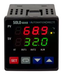
SOLO standard temperature controller, 1/16 DIN, 2-line LED, current, voltage, RTD or thermocouple input, 4-20 mA, 5A SPST relay, (2) 3A SPST relays output, 100-240 VAC operating voltage, RS-485.
