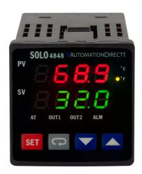
SOLO standard temperature controller, 1/16 DIN, 2-line LED, current, voltage, RTD or thermocouple input, 4-20 mA, 5A SPST relay, (2) 3A SPST relays output, 24 VDC operating voltage, RS-485.
