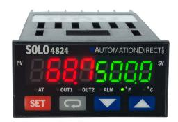
SOLO standard temperature controller, 1/32 DIN, 2-line LED, current, voltage, RTD or thermocouple input, (2) 3A SPST relays output, 24 VDC operating voltage, RS-485.
