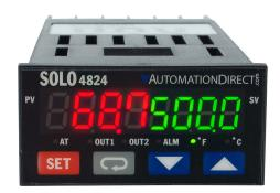
SOLO standard temperature controller, 1/32 DIN, 2-line LED, current, voltage, RTD or thermocouple input, 0-10VDC, 3A SPST relay output, 100-240 VAC operating voltage, RS-485.
