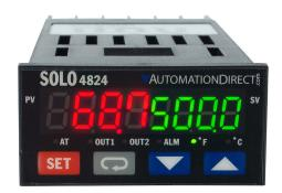
SOLO standard temperature controller, 1/32 DIN, 2-line LED, current, voltage, RTD or thermocouple input, 0-10 VDC, 3A SPST relay output, 100-240 VAC operating voltage, RS-485.
