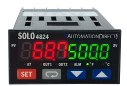
SOLO standard temperature controller, 1/32 DIN, 2-line LED, current, voltage, RTD or thermocouple input, 4-20 mA, 3A SPST relay output, 100-240 VAC operating voltage, RS-485.
