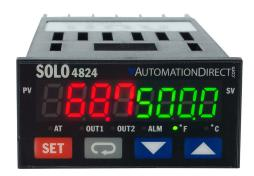
SOLO standard temperature controller, 1/32 DIN, 2-line LED, current, voltage, RTD or thermocouple input, 4-20 mA, 3A SPST relay output, 24 VDC operating voltage, RS-485.
