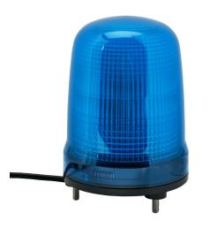
Patlite SL series LED industrial signal beacon, 150mm, blue, selectable continuous, blinking or triple flash, IP23, base mount, 12-24 VDC.
