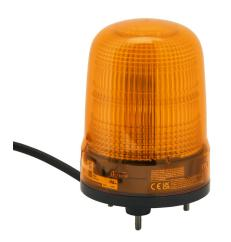
Patlite SL series LED industrial signal beacon, 100mm, amber, selectable continuous, blinking or triple flash, IP23, base mount, 100-240 VAC. IP65 when used with SZW-103 rubber gasket.
