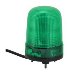
Patlite SL series LED industrial signal beacon, 100mm, green, selectable continuous, blinking or triple flash, IP23, base mount, 100-240 VAC. IP65 when used with SZW-103 rubber gasket.
