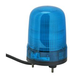
Patlite SL series LED industrial signal beacon, 100mm, blue, selectable continuous, blinking or triple flash, IP23, base mount, 100-240 VAC. IP65 when used with SZW-103 rubber gasket.
