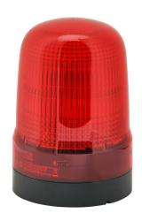
Patlite SL series LED audible-visual signal beacon, 88 dB at 1m, continuous tone(s), selectable continuous, blinking or triple flash, red, 100mm, 12-24 VDC, IP66, NEMA 4X/13, push-in terminal.
