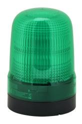
Patlite SL series LED audible-visual signal beacon, 88 dB at 1m, continuous tone(s), selectable continuous, blinking or triple flash, green, 100mm, 12-24 VDC, IP66, NEMA 4X/13, push-in terminal.
