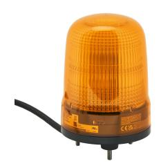
Patlite SL series LED industrial signal beacon, 100mm, amber, selectable continuous, blinking or triple flash, IP23, base mount, 12-24 VDC. IP65 when used with SZW-103 rubber gasket.
