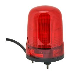
Patlite SL series LED industrial signal beacon, 100mm, red, selectable continuous, blinking or triple flash, IP23, base mount, 12-24 VDC. IP65 when used with SZW-103 rubber gasket.
