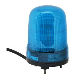
Patlite SL series LED industrial signal beacon, 100mm, blue, selectable continuous, blinking or triple flash, IP23, base mount, 12-24 VDC. IP65 when used with SZW-103 rubber gasket.
