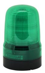
Patlite SL series LED audible-visual signal beacon, 86 dB at 1m, continuous tone(s), selectable continuous, blinking or triple flash, green, 80mm, 100-240 VAC, IP66, NEMA 4X/13, push-in terminal.
