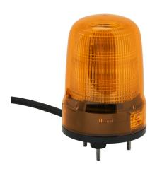
Patlite SL series LED industrial signal beacon, 80mm, amber, selectable continuous, blinking or triple flash, IP23, base mount, 100-240 VAC. IP65 when used with SZW-102 rubber gasket.
