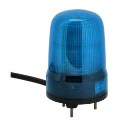
Patlite SL series LED industrial signal beacon, 80mm, blue, selectable continuous, blinking or triple flash, IP23, base mount, 100-240 VAC. IP65 when used with SZW-102 rubber gasket.
