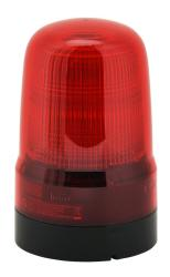
Patlite SL series LED audible-visual signal beacon, 86 dB at 1m, continuous tone(s), selectable continuous, blinking or triple flash, red, 80mm, 12-24 VDC, IP66, NEMA 4X/13, push-in terminal.
