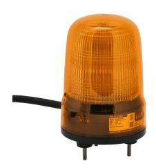
Patlite SL series LED industrial signal beacon, 80mm, amber, selectable continuous, blinking or triple flash, IP23, base mount, 12-24 VDC. IP65 when used with SZW-102 rubber gasket.
