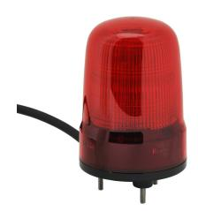
Patlite SL series LED industrial signal beacon, 80mm, red, selectable continuous, blinking or triple flash, IP23, base mount, 12-24 VDC. IP65 when used with SZW-102 rubber gasket.
