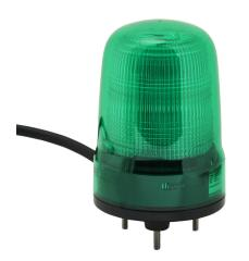
Patlite SL series LED industrial signal beacon, 80mm, green, selectable continuous, blinking or triple flash, IP23, base mount, 12-24 VDC. IP65 when used with SZW-102 rubber gasket.
