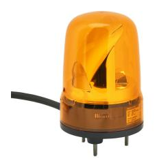
Patlite SK series LED industrial signal beacon, 80mm, amber, rotating (120rpm), IP23, base mount, 100-240 VAC. IP65 when used with SZW-102 rubber gasket.
