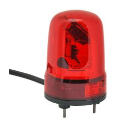
Patlite SK series LED industrial signal beacon, 80mm, red, rotating (120rpm), IP23, base mount, 100-240 VAC. IP65 when used with SZW-102 rubber gasket.
