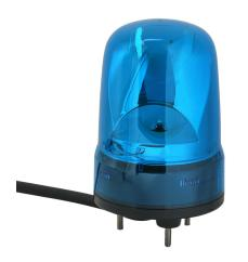
Patlite SK series LED industrial signal beacon, 80mm, blue, rotating (120rpm), IP23, base mount, 100-240 VAC. IP65 when used with SZW-102 rubber gasket.
