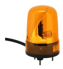
Patlite SK series LED industrial signal beacon, 80mm, amber, rotating (120rpm), IP23, base mount, 12-24 VDC. IP65 when used with SZW-102 rubber gasket.
