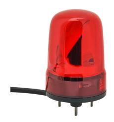
Patlite SK series LED industrial signal beacon, 80mm, red, rotating (120rpm), IP23, base mount, 12-24 VDC. IP65 when used with SZW-102 rubber gasket.
