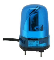
Patlite SK series LED industrial signal beacon, 80mm, blue, rotating (120rpm), IP23, base mount, 12-24 VDC. IP65 when used with SZW-102 rubber gasket.
