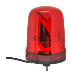
Patlite SK series LED industrial signal beacon, 150mm, red, rotating (120rpm), IP23, base mount, 100-240 VAC.
