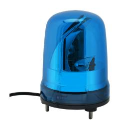
Patlite SK series LED industrial signal beacon, 150mm, blue, rotating (120rpm), IP23, base mount, 12-24 VDC.
