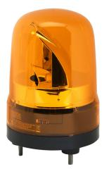
Patlite SK series LED audible-visual signal beacon, 88 dB at 1m, intermittent tone(s), rotating (120rpm), amber, 100mm, 100-240 VAC, IP23, push-in terminal.
