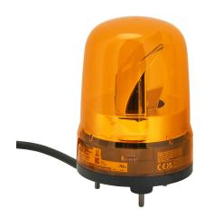
Patlite SK series LED industrial signal beacon, 100mm, amber, rotating (120rpm), IP23, base mount, 100-240 VAC. IP65 when used with SZW-103 rubber gasket.
