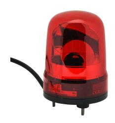
Patlite SK series LED industrial signal beacon, 100mm, red, rotating (120rpm), IP23, base mount, 100-240 VAC. IP65 when used with SZW-103 rubber gasket.
