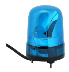
Patlite SK series LED industrial signal beacon, 100mm, blue, rotating (120rpm), IP23, base mount, 100-240 VAC. IP65 when used with SZW-103 rubber gasket.
