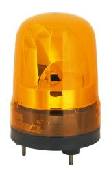
Patlite SK series LED audible-visual signal beacon, 88 dB at 1m, intermittent tone(s), rotating (120rpm), amber, 100mm, 12-24 VDC, IP23, push-in terminal.
