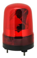
Patlite SK series LED audible-visual signal beacon, 88 dB at 1m, intermittent tone(s), rotating (120rpm), red, 100mm, 12-24 VDC, IP23, push-in terminal.
