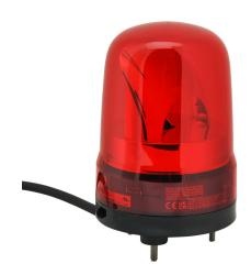
Patlite SK series LED audible-visual signal beacon, 88 dB at 1m, intermittent tone(s), rotating (120rpm), red, 100mm, 12-24 VDC, IP23, pigtail.
