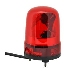
Patlite SK series LED industrial signal beacon, 100mm, red, rotating (120rpm), IP23, base mount, 12-24 VDC. IP65 when used with SZW-103 rubber gasket.
