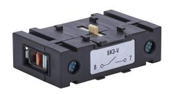
Merz fourth pole module, 600 VAC, 125A, load break capable, 5kA SCCR, UL 508 rated. For use with Merz ML3 switch bodies in DIN rail applications.
