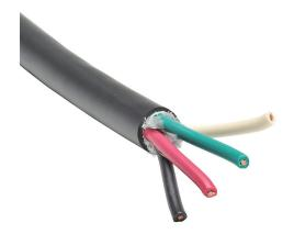
Southwire portable cord, unshielded, SJOOW, 300V, 4 conductors (includes ground), 18 AWG, EPDM thermoset rubber conductor insulation material, black, white, red and green, CPE thermoset rubber jacket, black, cut to length.
