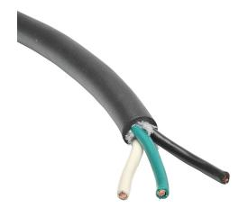
Southwire portable cord, unshielded, SJOOW, 300V, 3 conductors (includes ground), 18 AWG, EPDM thermoset rubber conductor insulation material, black, white and green, CPE thermoset rubber jacket, black, cut to length.
