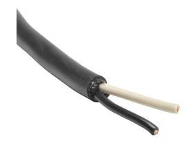
Southwire portable cord, unshielded, SJOOW, 300V, 2 conductors, 18 AWG, EPDM thermoset rubber conductor insulation material, black and white, CPE thermoset rubber jacket, black, cut to length.
