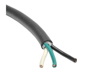
Southwire portable cord, unshielded, SJOOW, 300V, 3 conductors (includes ground), 16 AWG, EPDM thermoset rubber conductor insulation material, black, white and green, CPE thermoset rubber jacket, black, cut to length.
