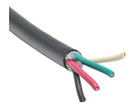
Southwire portable cord, unshielded, SJOOW, 300V, 4 conductors (includes ground), 14 AWG, EPDM thermoset rubber conductor insulation material, black, white, red and green, CPE thermoset rubber jacket, black, cut to length.
