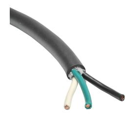
Southwire portable cord, unshielded, SJOOW, 300V, 3 conductors (includes ground), 14 AWG, EPDM thermoset rubber conductor insulation material, black, white and green, CPE thermoset rubber jacket, black, cut to length.
